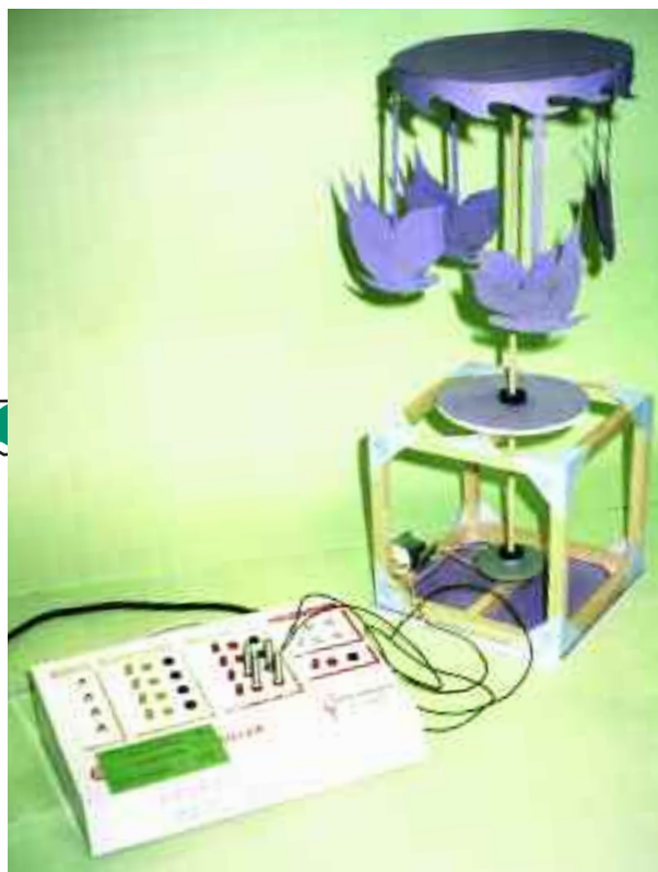
Fairground carousel being controlled by a computer linked to the model through an interface / control box
