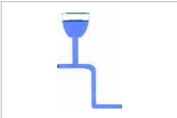
Double-variation task: pipe-end height (higher pipe-end-less flow) and resistance to end (longer pipe – more resistance – less flow)
