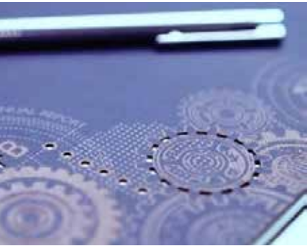
Adjusting power settings will achieve different cutting and engraving results. This example shows a piece of card which has been cut and engraved with varying degrees of intensity and detail.
