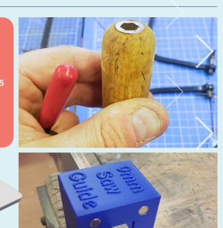
into the end of the coping saw and give the students the support that they need. Once we have supported the students to cut their work, we can quickly unscrew the handle and work our way around the group. We've already expanded this idea and added extra handles to tenon saws and seen more positive results in student confidence and skills.
